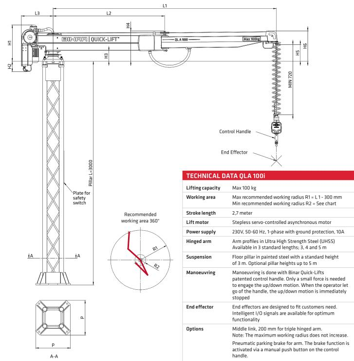
Middle link and pneumatic parking brake can not be combined.
