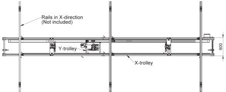
The rail system, Quick-Lift Driven 300i (QLD 300i) is a unique, motorized lifting device that easily covers large areas horizontally, with a lifting load up to 300 kg.
